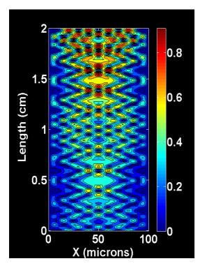
Silicon Image Amplifier. A pixilated image is simultaneously amplified and imaged as it propagates through a multimode waveguide (vertical axis represents the propagation direction).
